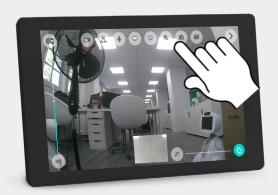
The zoom video camera (80°) is now active, and the user can continue to pilot the robot, positioning the head in the area where he wishes to take a photo and save it in the gallery.
