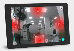
A red indicator is displayed when the robot hits an obstacle while moving forward or backward.
